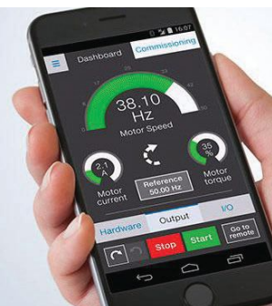
Figure 1: The ability to connect a smartphone to one or more variable frequency drives (VFDs) through Bluetooth is one of the recent developments that have made the operation of drives easier and safer. All images courtesy: ABB Inc.
